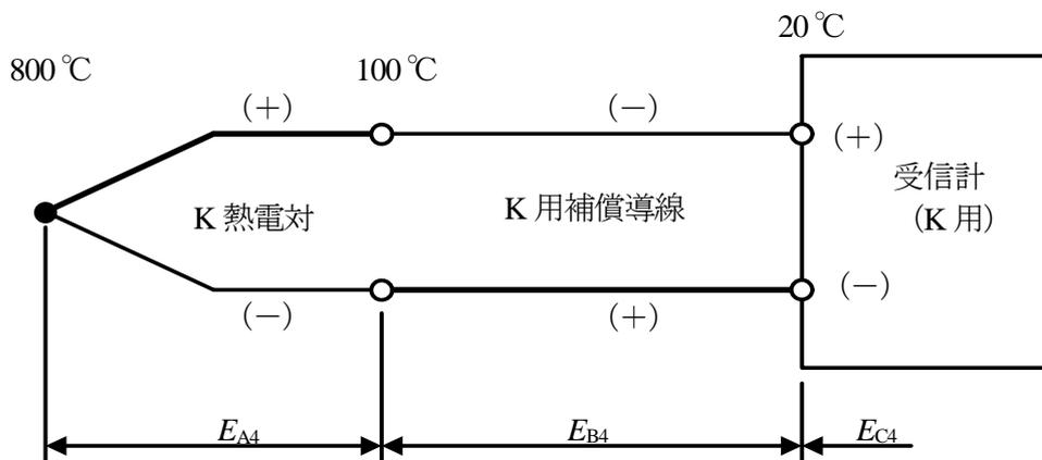
$$E_{A4} + E_{B4} + E_{C4} = (33\,275 - 4\,096)\ \mu\text{V} - (4\,096 - 798)\ \mu\text{V} + 798\ \mu\text{V} \\ = 26\,679\ \mu\text{V}$$
